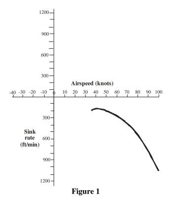
In this case the sink rate was noted for 5-knot airspeed intervals from stall in the clean configuration to 100 knots. The left end of the curve is the stall airspeed, and the right end is the highest airspeed evaluated ( $V_{NE}$  for this aircraft is 124 kt).
